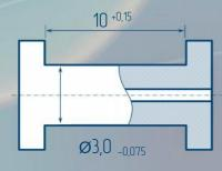
5000 turns, wire Ø0,063 mm coil resistance 580
